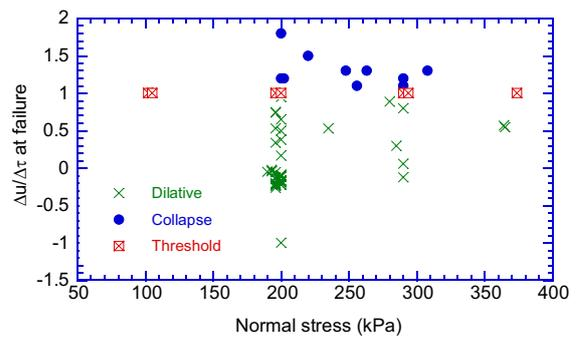
Fig. 1 The boundary between contraction and dilation
