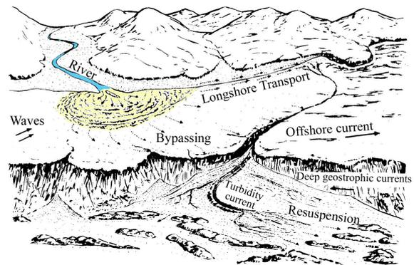
Fig. 1 Schematic of sediment routing system (adapted from Seibold and Berger, 1993)
