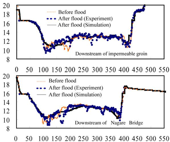
Fig. 14 Evolution of cross-channel profiles (Zhang et al, 2007b)
