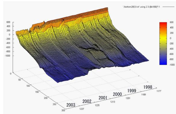
Fig. 19 A snapshot of the measured evolution of seabed profile along the observation pier
