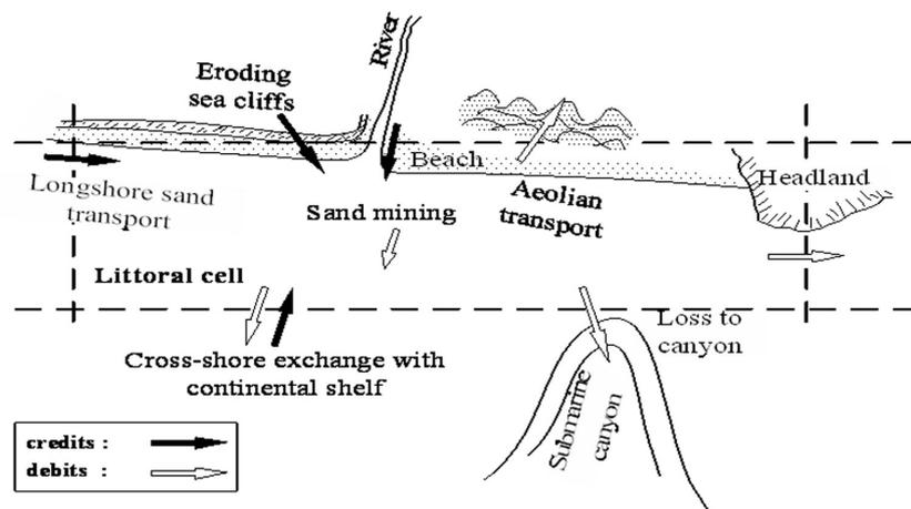
Fig. 15 Principal components involved in the development of a budget of littoral sediment (adapted from Komar, 1998)
