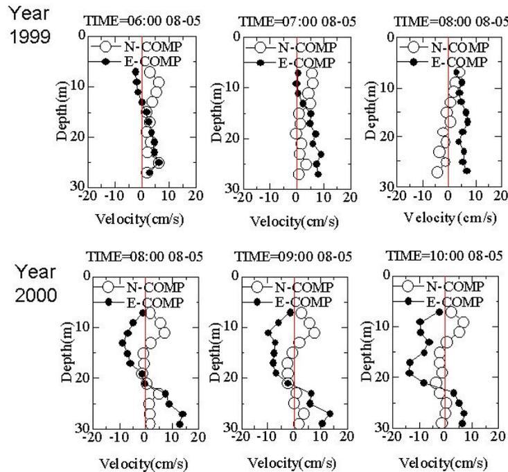
Fig. 24 Observed profiles of flow velocities of seawater
