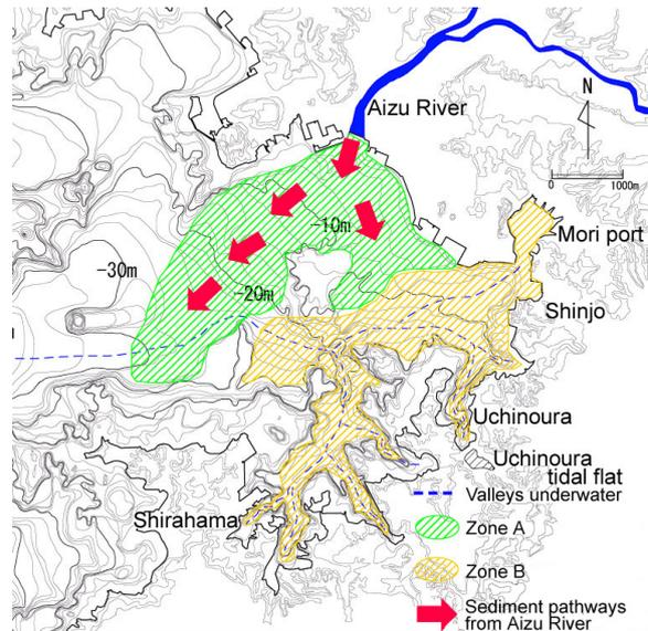
Fig. 29 Identification of distributions of coarse-grained sediment (zone A) and fine-grained sediment (zone B)
