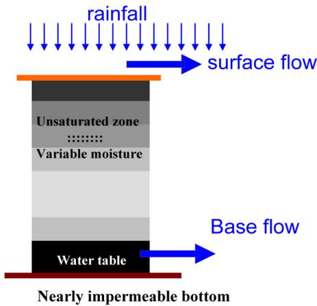
Fig. 3 Surface and base flows in grid-based model
