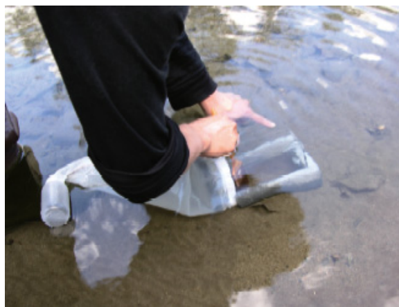
Photo 2 A BPOM sampler under operation in the field.
