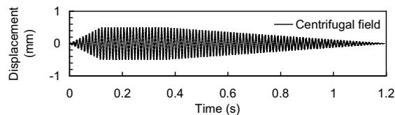
Fig. 3 Example of input displacement in centrifugal field.
