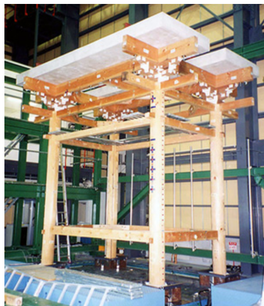
Photo 1 Shaking table test of specimen
