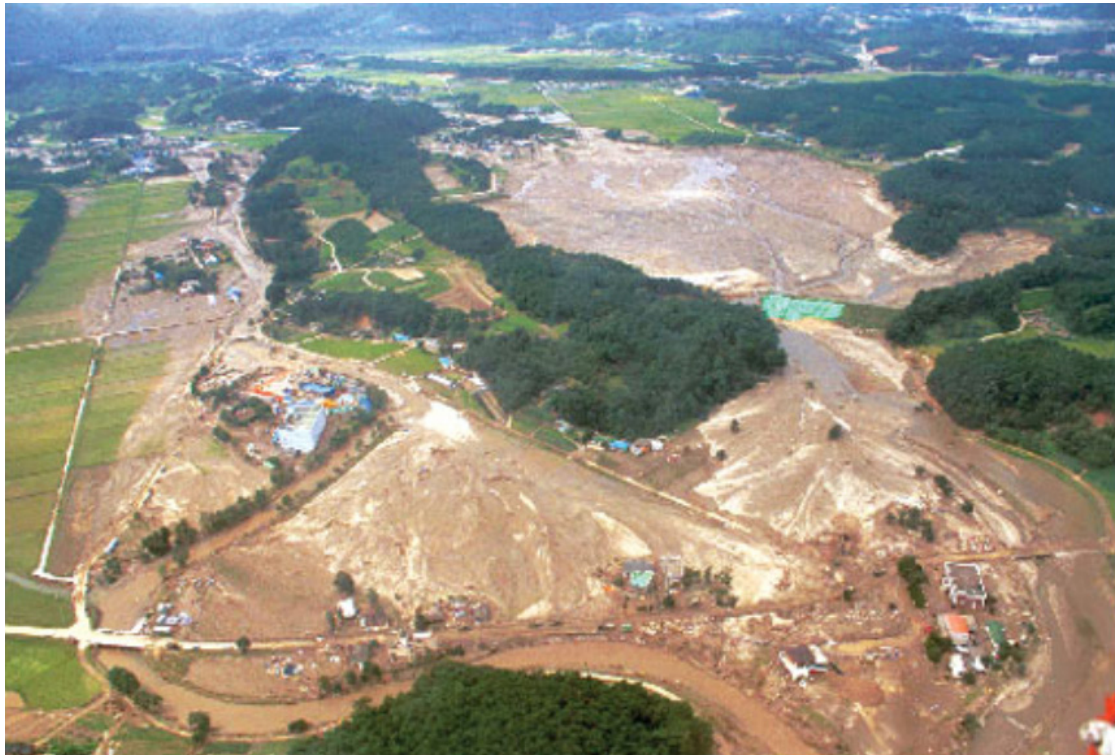
Fig. 2 JangHyun reservoir breached and swept a whole village during Typhoon Rusa
