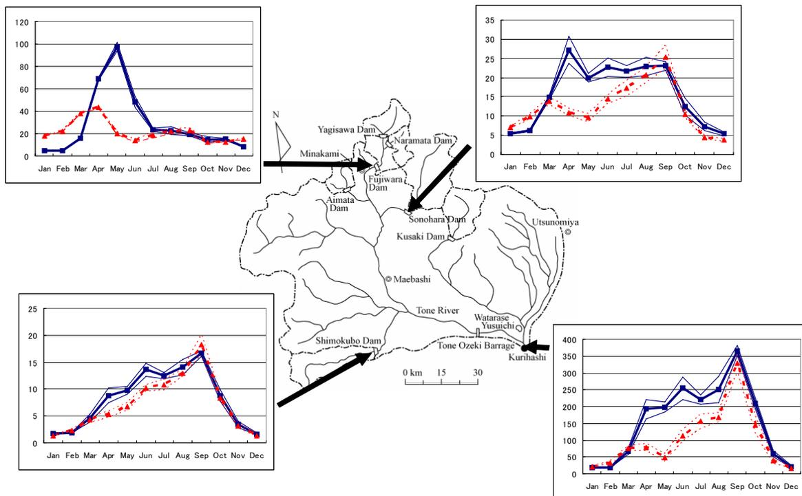
Fig. 9 The flow discharges at the Fujiwara Dam, Simokubo Dam, Sonohara Dam and Kurihashi. See Fig.8 for the line legends.
