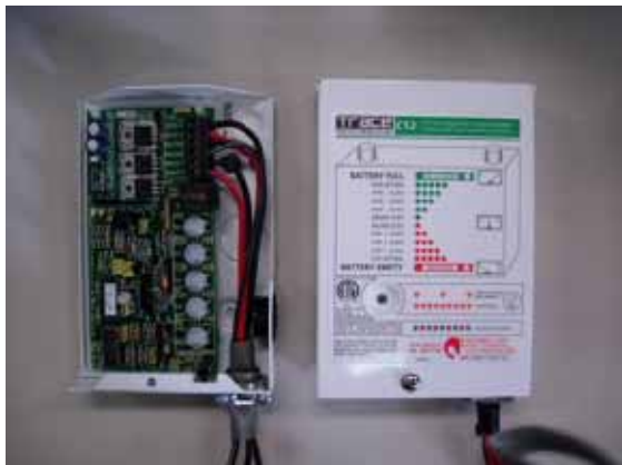
c. Controller of solar panel (C12)
