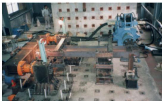
Fig. 7 Test setup for full-scale steel beam
