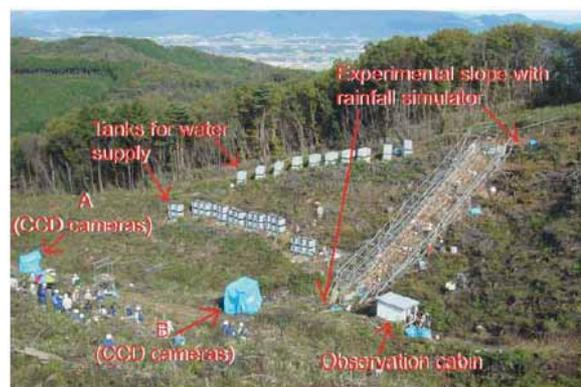
Fig. 19 View of the experiment site at Mt. Kaba-san.
