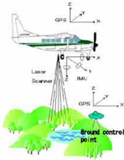
Fig. 4 Measuring principle of airborne laser scanning
