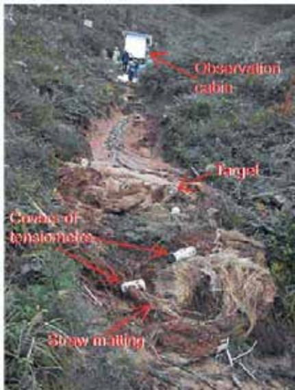
Fig. 21 The landslide deposit one day after the experiment.
