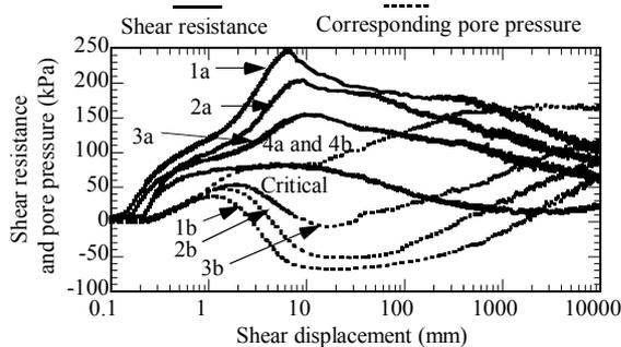
Fig. 8 Shear resistances and the corresponding pore pressures of some sands as density changes (specimens at 196kPa confining stress)
