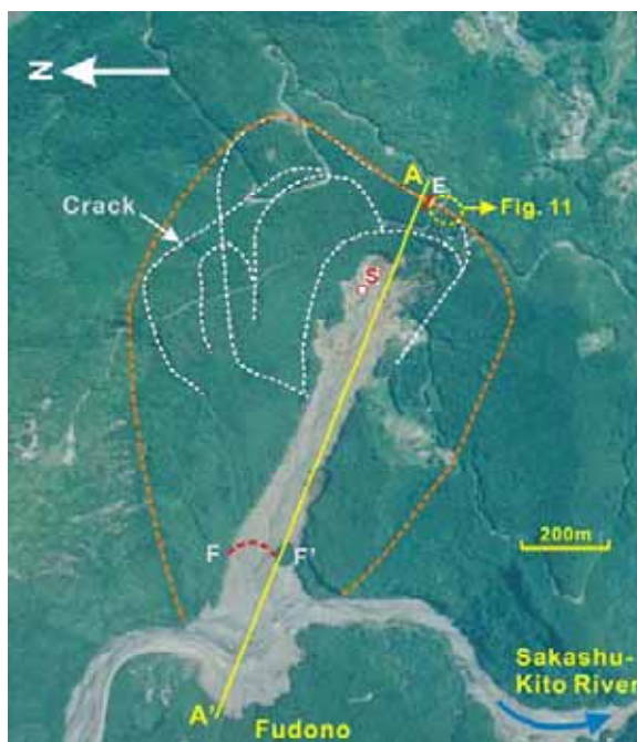
Photo 5 Oblique aerial view of Azue landslide and the unstable blocks after the August 1, 2004 event (photo by Nakanihon Sky Service Station, Japan). The broken brown line outlines the area of the ancient landslide
