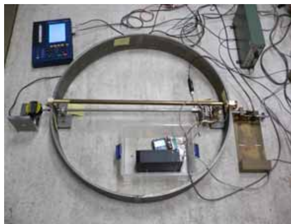
Photo 1 Calibration of the short span strainmeter by using a device with screw.
