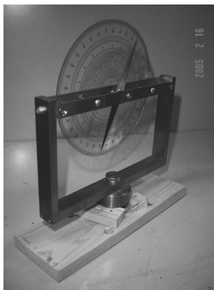
Photo 1 The dip circle used in this study.
