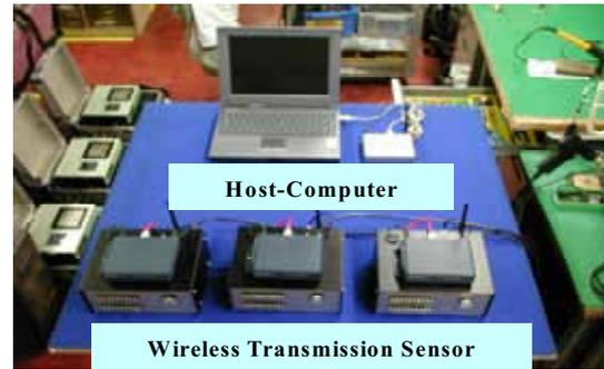
Fig.9 Wire less data acquisition system
