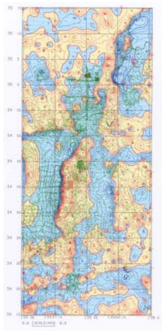
Fig.2 Residual Bouguer anomaly filtered with upward continuation (50m - 5,000m). Contour interval = 1\text{mGal} .
