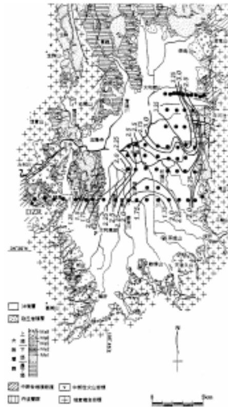
Fig. 8 Peak period of H/V spectral ratio of microseisms. Contour interval = 0.25s. After Morikawa et al.(1998).
