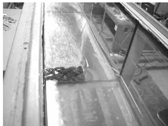
Photo 7 Laboratory experiment on rubble mound groin (Case-B, i.e. h > h_g ).
