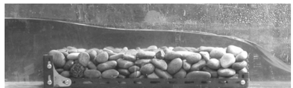
Photo 4 An experimental setup for flow over a rubble mound weir.
