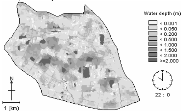
Fig.33 The inundation water depth after 22 hours
