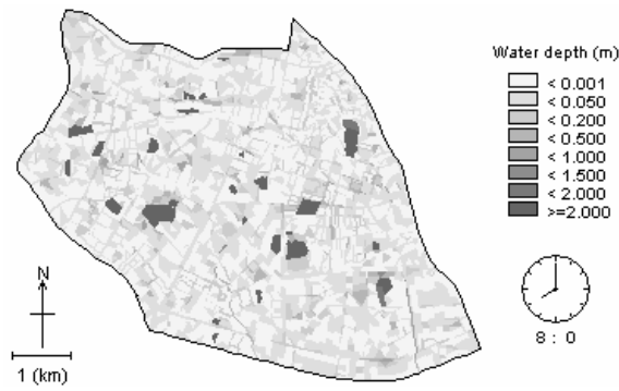
Fig.31 The inundation water depth after 8 hours
