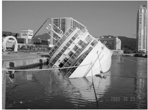
Photo.4 Damage of the floating hotel
