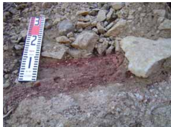
Fig. 6 Slip zone of the landslide M-1. A red band is seen in the middle of the pictures. It is made within the weathered tuff breccia, which had been oxidated beneath the overlying autobrecciated lava.
