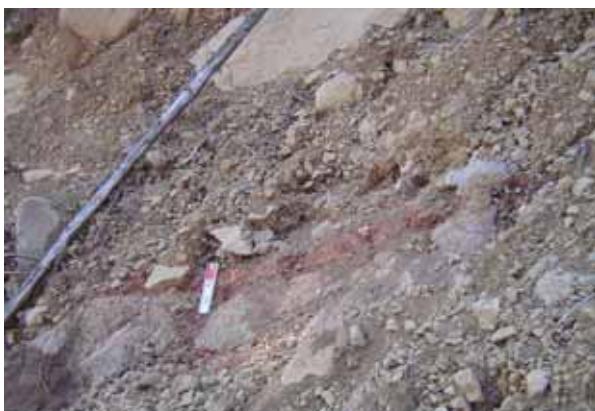
Fig. 6 Slip zone of the landslide M-1. A red band is seen in the middle of the pictures. It is made within the weathered tuff breccia, which had been oxidated beneath the overlying autobrecciated lava.
