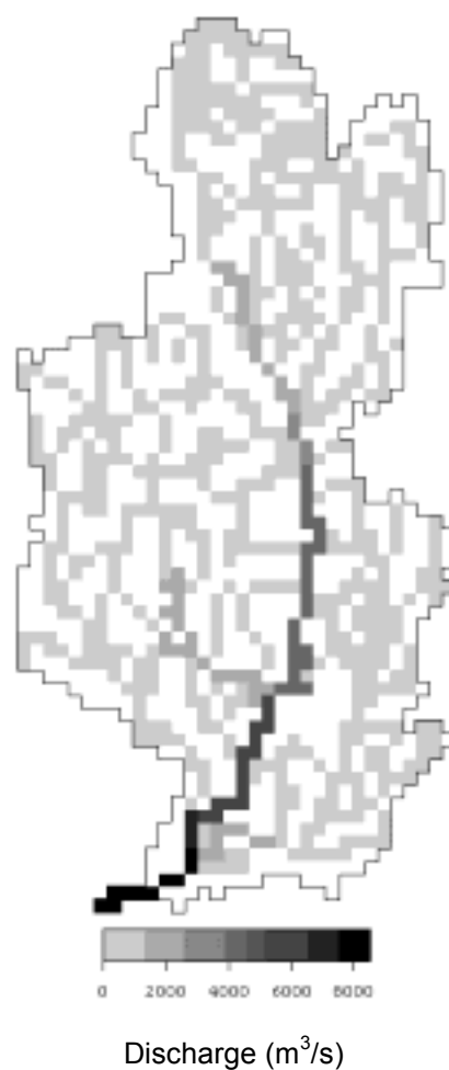
Fig. 9 Distributed discharge forecast for the Nagara River watershed, 6-hours ahead, (a) 50% non-exceedance probability limit (left), (b) 95% non-exceedance probability limit (right), 20:00 11 September 2000
