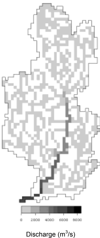
Fig. 9 Distributed discharge forecast for the Nagara River watershed, 6-hours ahead, (a) 50% non-exceedance probability limit (left), (b) 95% non-exceedance probability limit (right), 20:00 11 September 2000
