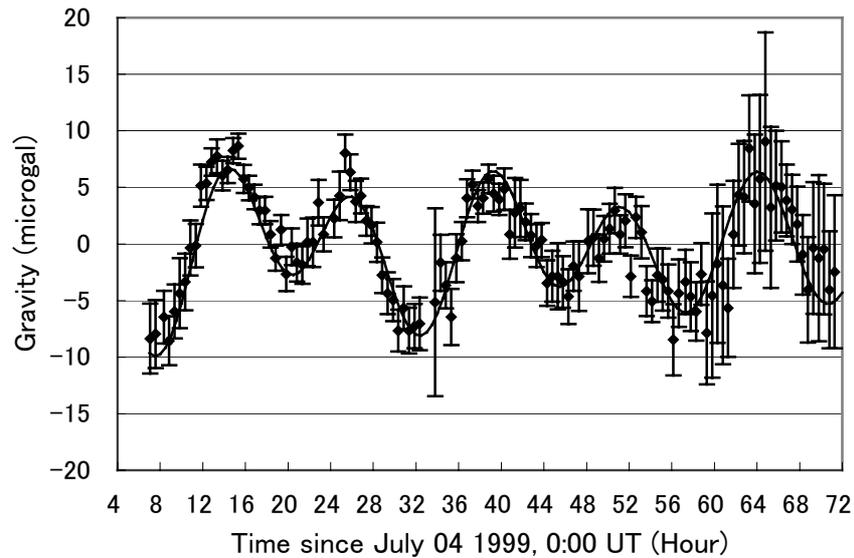
Fig. 2 The FG5 record observed at SVO in July 1999 (Solid diamonds with error bars). The absolute gravity values after correcting for solid earth tide, pole tide and barometric effects are plotted with respect to a value of 979,451,835.4  $\mu\text{gal}$ . Solid curves are the theoretical ocean tides calculated by GOTIC2.
