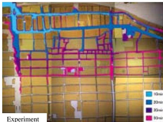
Fig.13 Comparison between flooded area in experiment and that in calculation (intrusion into underground space is considered)
