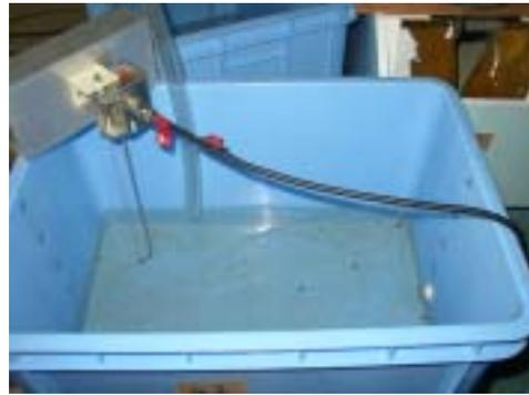
Fig. 4: Capacity type water gauge
