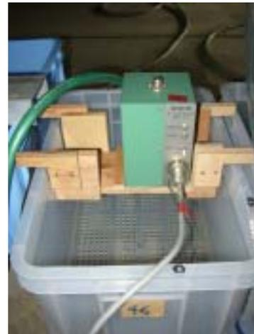
Fig. 5: Servo type water gauge
