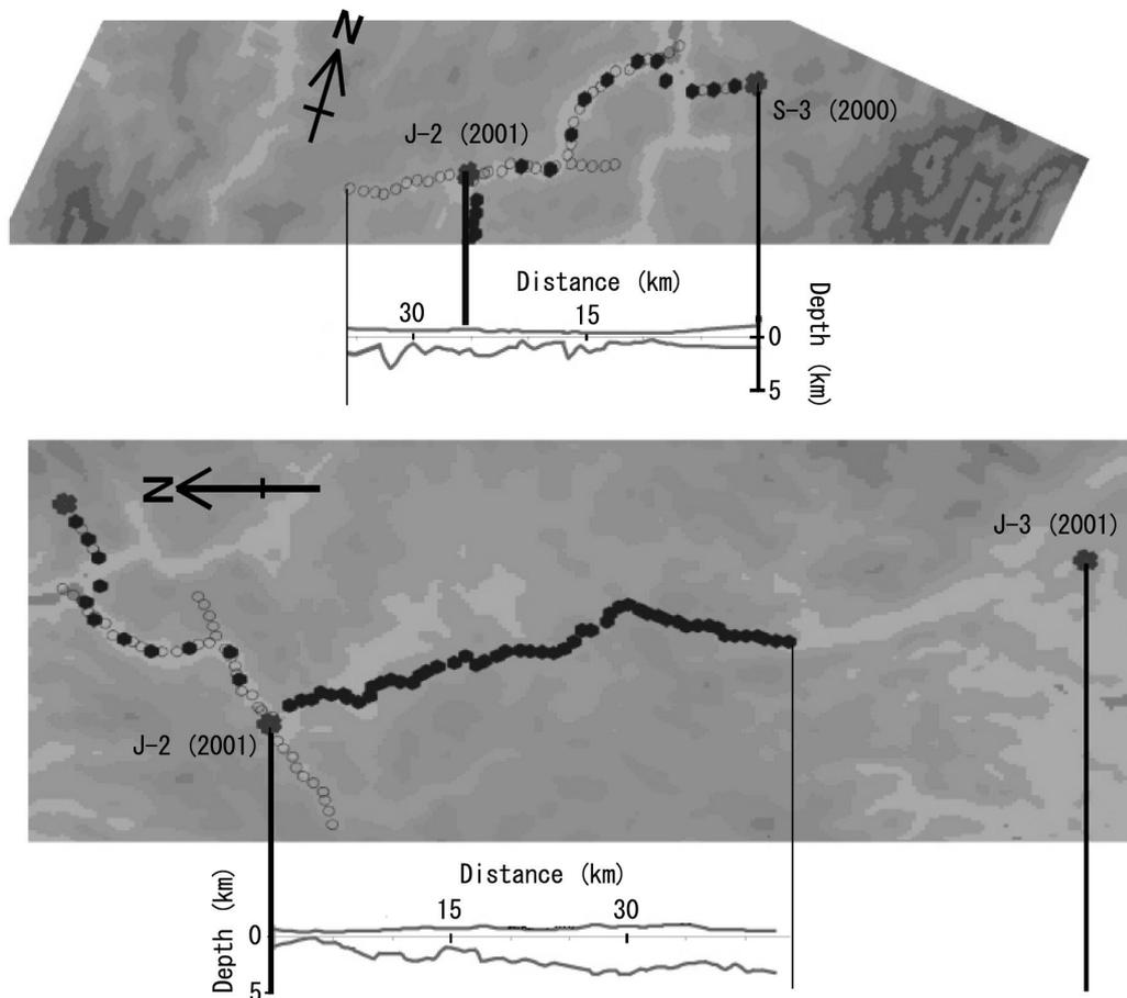
Fig. 3 Locations of shots and stations, and depth of surface layer along (upper figure) and perpendicular to (lower figure) the Atotsugawa fault system. Depths are calculated from the time-terms on the assumption of the velocities of the surface layer and basement to be 4.5 and 5.9 km/s.
