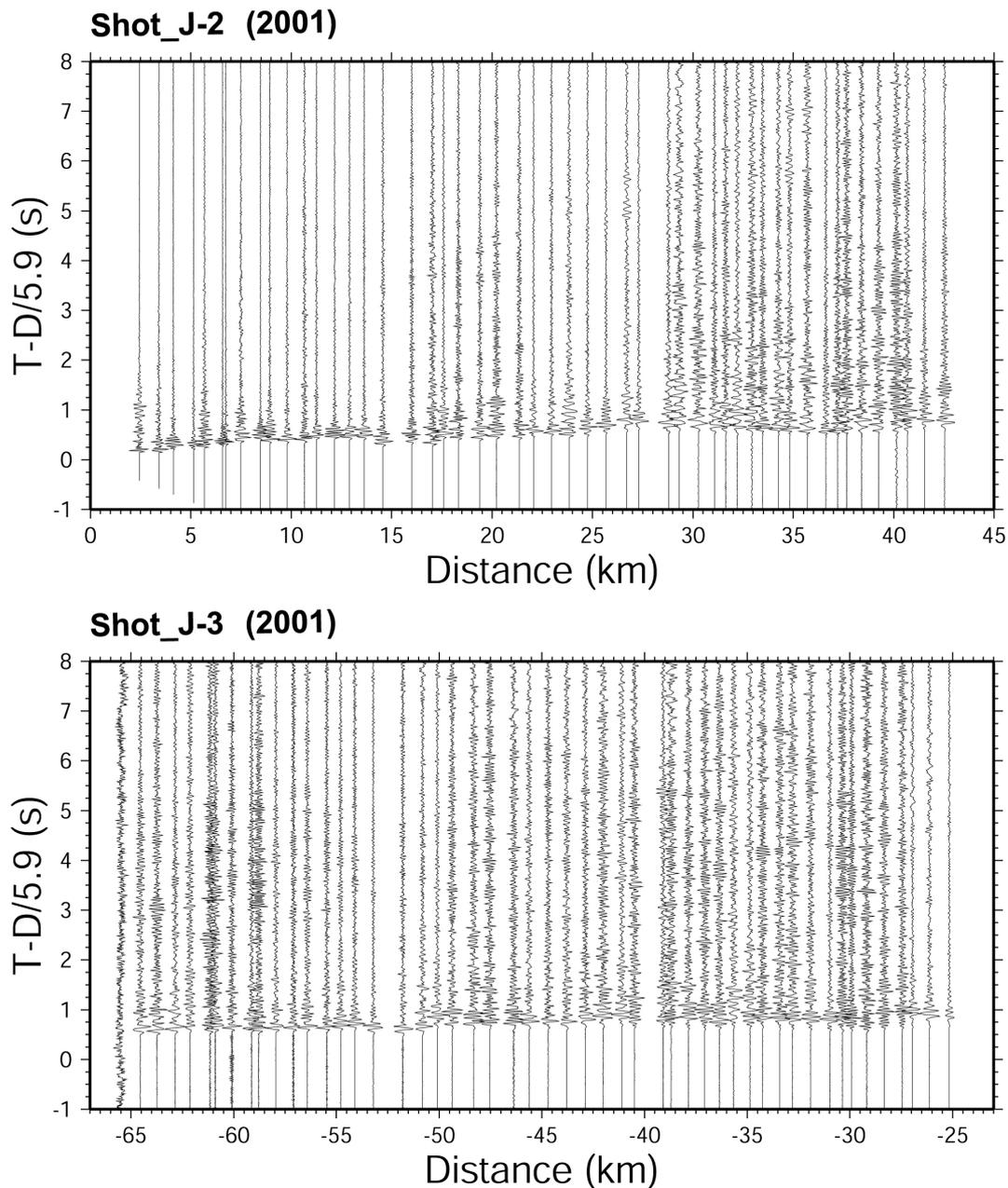
Fig. 2-2. Record sections of the shots J-2 (upper figure) and J3 (lower figure) in 2001 perpendicular to the Atotsugawa fault system.
