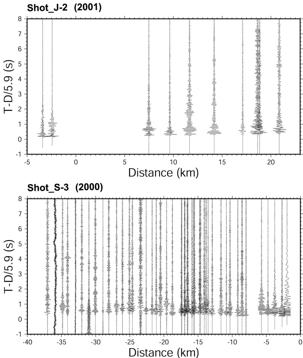
Fig. 2-1. Record sections of the shot J-2 in 2001 (upper figure) and shot S-3 in 2000 (lower figure) along the Atotsugawa fault system. Lower figure is reproduced after Yoshii et al. (2000).
