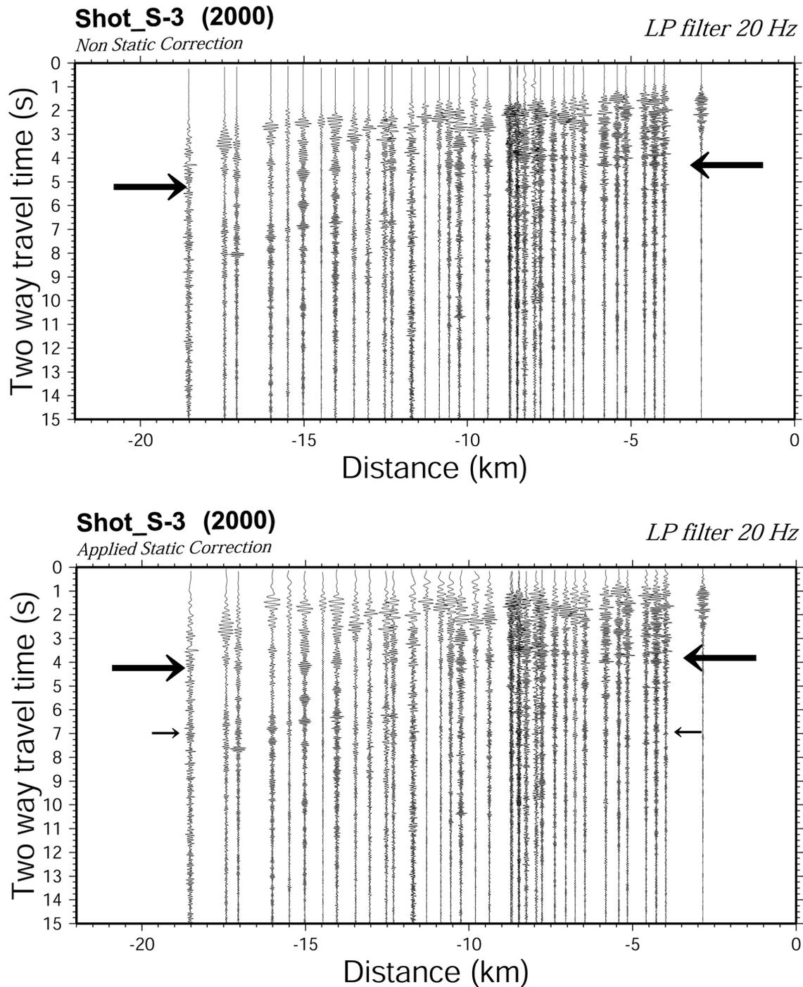
Fig. 4-1. NMO (normal-move-out) corrected record sections for S-3 without (upper figure) and with (lower figure) static correction. Low-pass filter (20 Hz) is applied.
