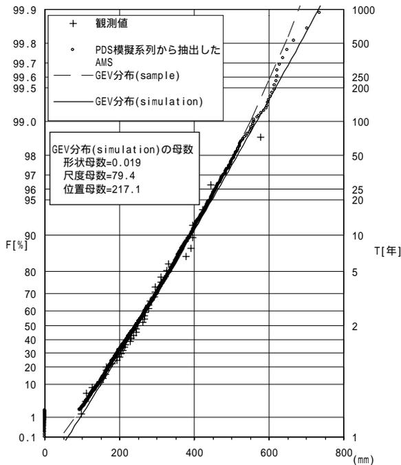
Fig. 11 An example of GEV distributions applied to observed AMS and extracted AMS from generated PDS (Inter event time: exponential distribution)
