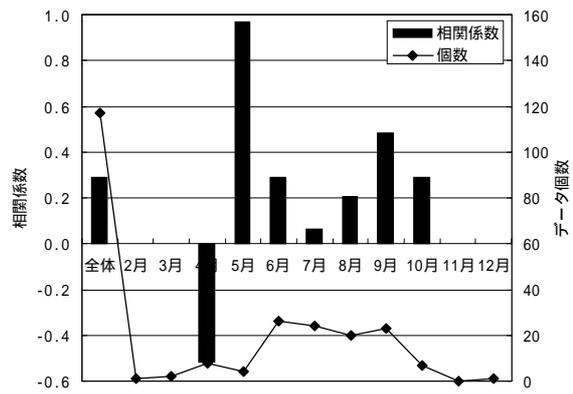
Fig. 9 Correlation coefficient between inter event time and peak discharge
