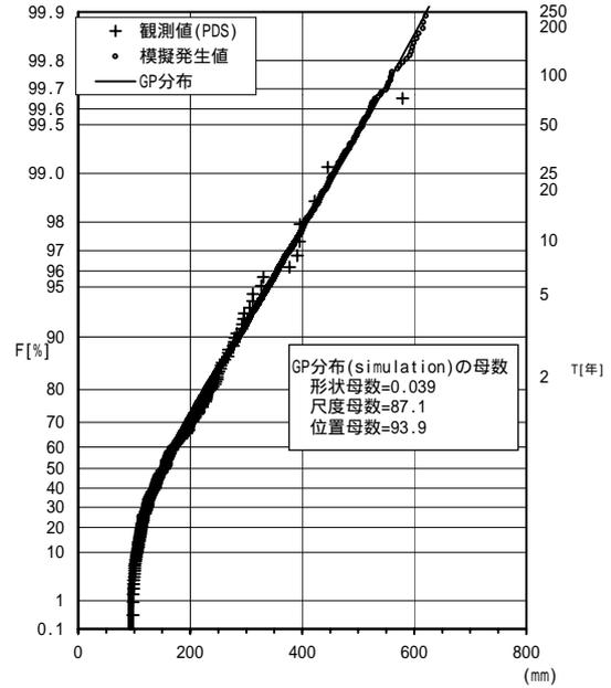
Fig. 10 Observed PDS and GP distribution applied to it (10000 PDS generated by the distribution are also shown)
