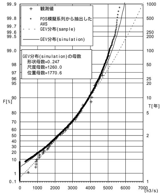
Fig. 18 An example of GEV distributions applied to observed AMS and extracted AMS from generated PDS (Inter event time: exponential distribution)
