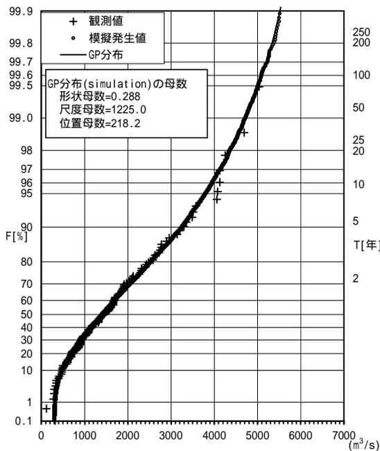
Fig. 17 Observed PDS and GP distribution applied to it (10000 PDS generated by the distribution are also shown)
