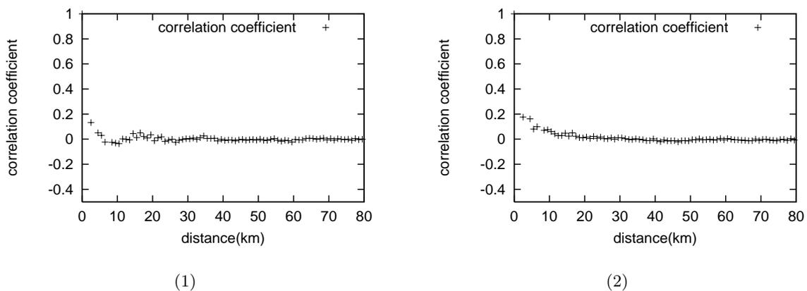
Fig. 5 Spatial correlation coefficient of relative prediction error  $E_r$ . (1) Case for 5 minute ahead prediction. (2) Case for 60 minute ahead prediction.
