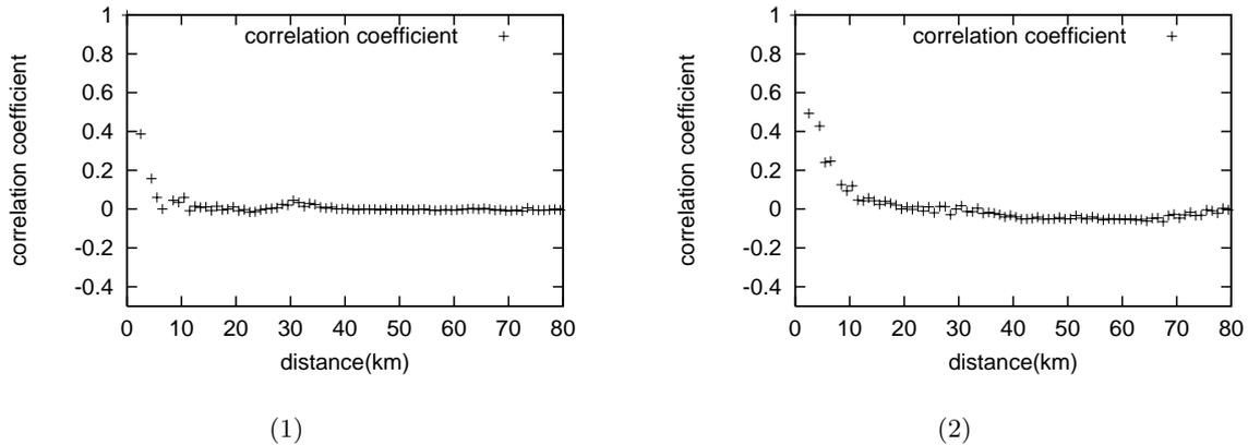
Fig. 3 Spatial correlation coefficient of prediction error  $E_a$ . (1) Case for 5 minute ahead prediction. (2) Case for 60 minute ahead prediction.
