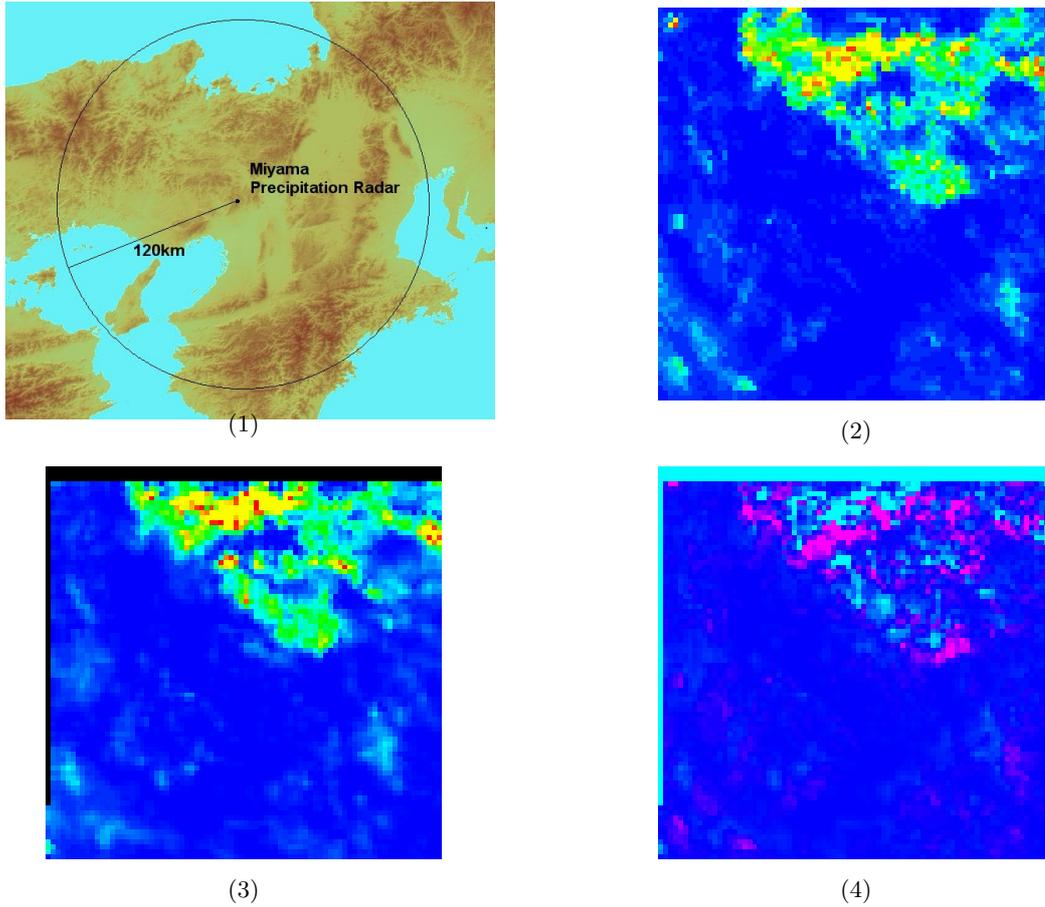
Fig. 1 (1) Quantitative measurement area by the Miyama precipitation radar (120km radius). (2) Observed rainfall by the Miyama radar at 0:15pm, September 5 in 1989. (3) 15 minute ahead rainfall prediction by the transration model (predicted at 0:00pm, September 5 in 1989). (4) Prediction error calculated as observed minus predicted value.
