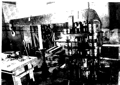
Fig. 1 Weight-lever type compression machine (150 kN) designed by T. Shida and M. Matsuyama in 1918
