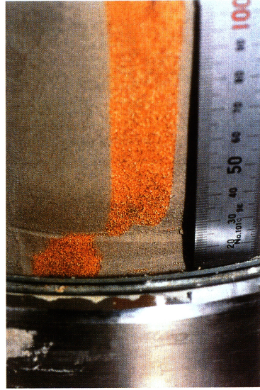
Fig. 11 Shear deformation of vertically inserted slice of Toyoura sand in the complementary test for the dense sand shown in Fig. 4 ( B_D = 0.99 ; D_r = 94.9\% ).
