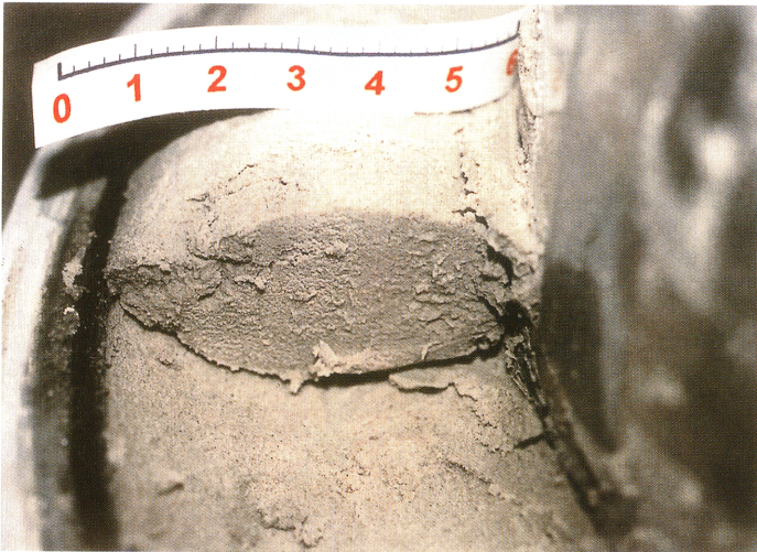
Fig. 12 Formation of shear zone for the tests on S8. (a): in loose state ( D_r = 63.3\% ; Shear displacement = 10 m); (b): in dense state ( D_r = 95.2\% ; Shear displacement = 210 m)
