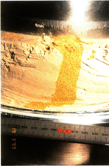
Fig. 10 Shear deformation of vertically inserted slice of Toyoura sand after 3-cm shear for the CT test shown in Fig. 9 ( B_D = 0.99 , D_r = 63.3\% ).
