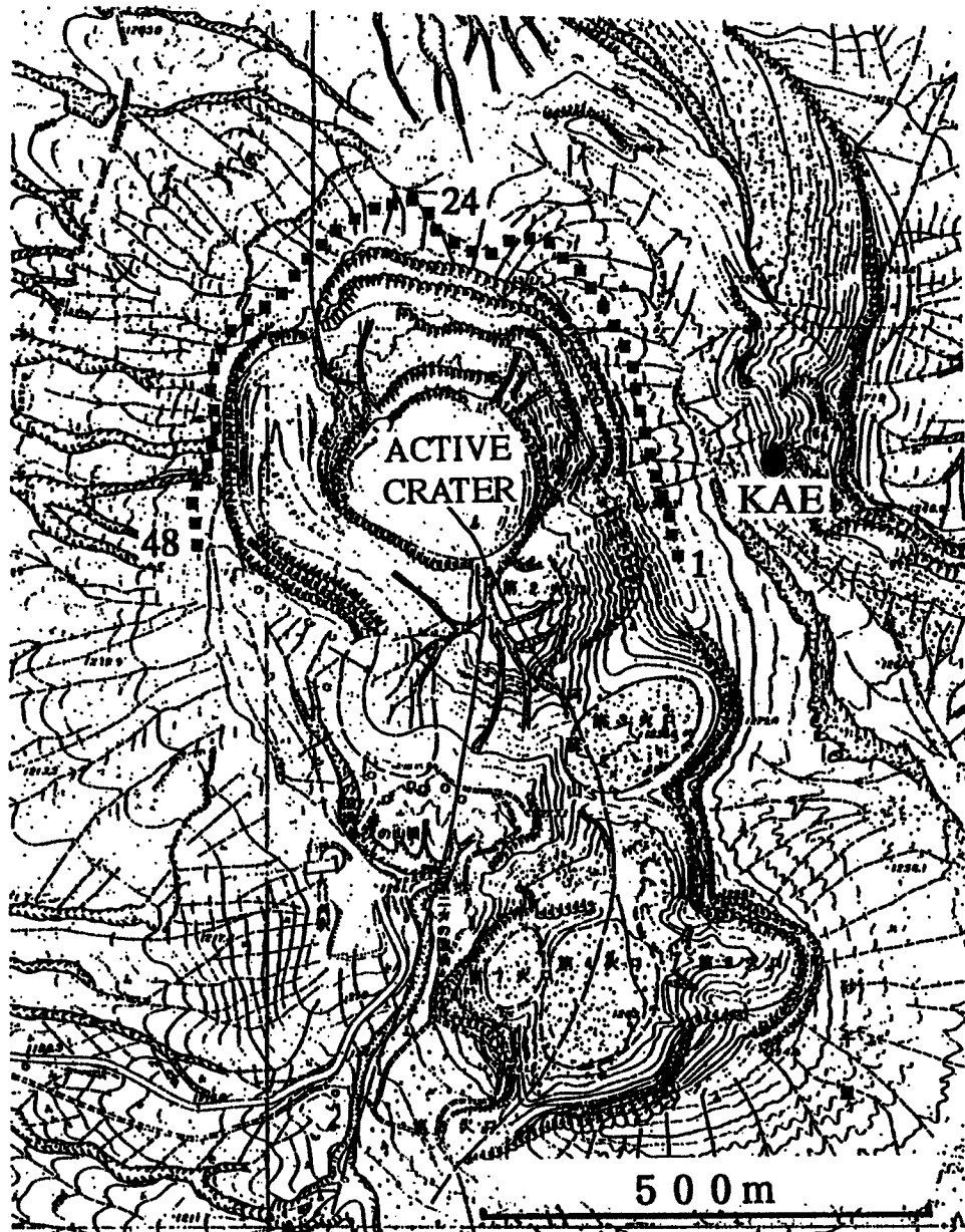
Fig. 3. A dense seismic array network used in this study of Aso Volcano around active crater (■: The dense network, ●: permanent station)
