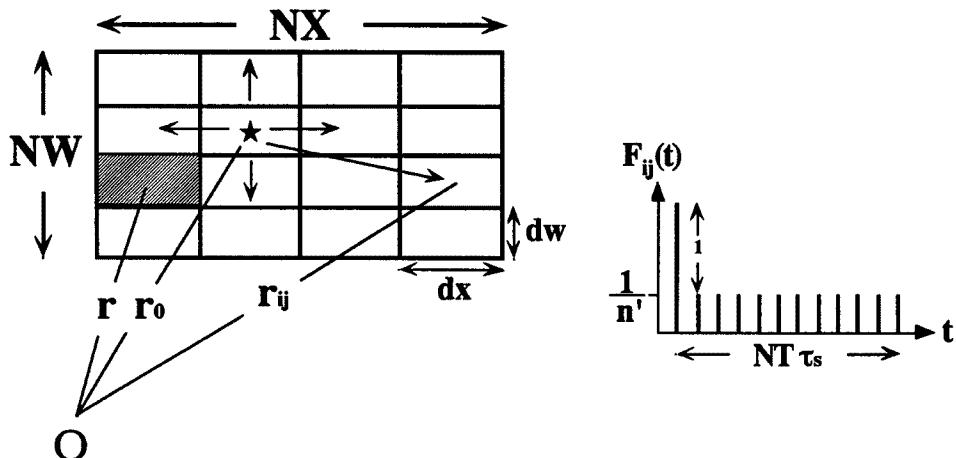
Fig. 3 Left: Schematic fault model for simulating seismograms.  $r_0$  is the hypocentral distance of the large event,  $r$  is that of the small event, and  $r_{ij}$  is the distance between the  $(i, j)$  subfault on the fault plane of the large event and the observation station. Right: The transfer function for correcting the difference in slip velocity time function between the large and small events.
