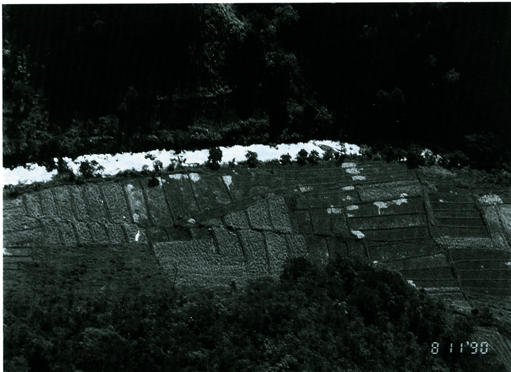
Photo 4. Aerial view toward the east showing left-lateral offset of the paddy field north of Imugan. An estimated offset is about 5 m.
