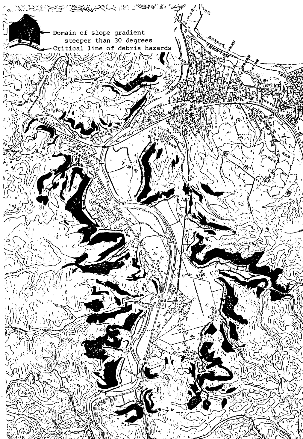
Fig. 17. Hazard area by slope failure predicted.
