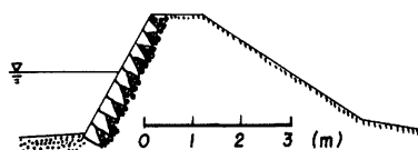
Fig. 16 Masonry breakwater at Obama coast, Omuta, Kyushu island in about 1890s.
