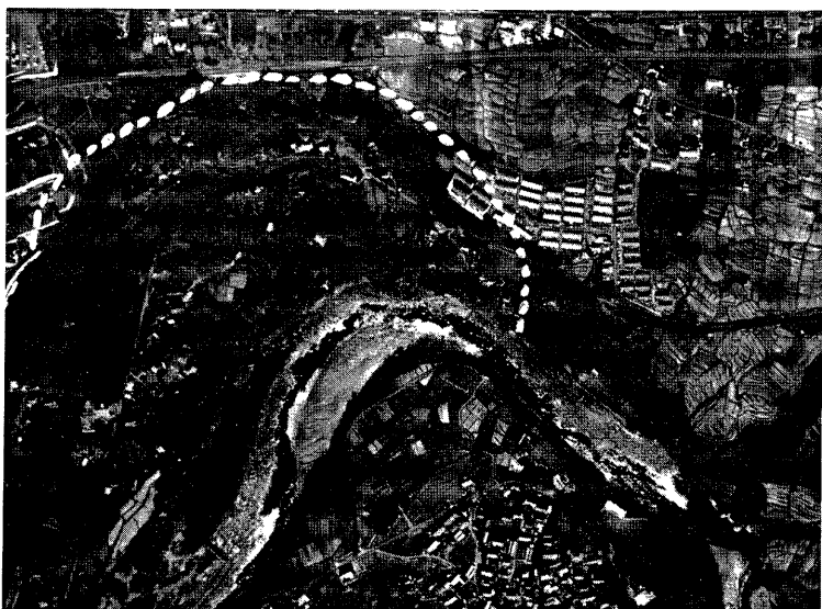
Photo. 2 The aerophotograph of the Oshidashi landslide and around the active area. The enclosed part with the broken line showed the active landslide area (accepted an offer by S. Hatano).
