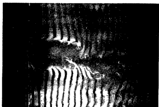
Photo. 13 Flow pattern around cylinder ( B/D = 1 , Re = 6.3 \times 10^3 , k = 2 St ).
