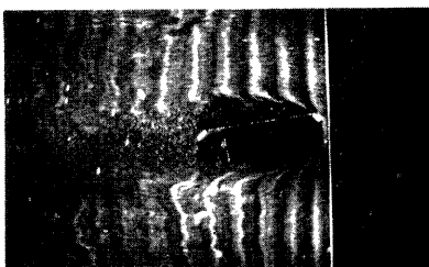
Photo. 6 Flow pattern (1:3 with Upper Deflector \alpha = 9^\circ )
