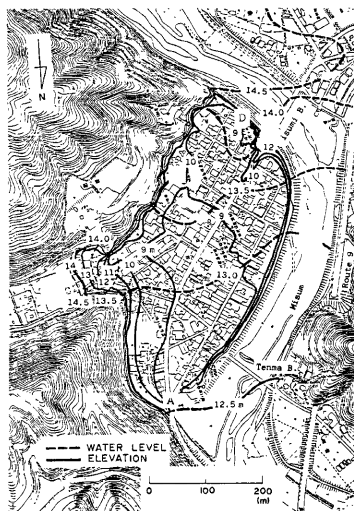
Fig. 3 Distribution of altitude and observed inundated water level in Misumi district
