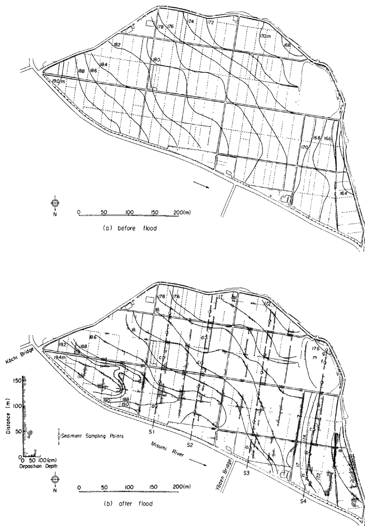
Fig. 14 Distributions of deposition depth of sediment on flood plain in Shimokōchi
