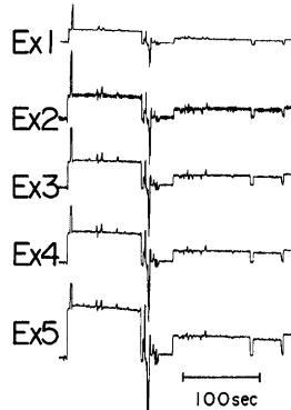
Fig. 11. Examples of wave form to determine relative sensitivities recorded after the Samoa Is. earthquake and SE off nemuro Pen. earthquake. Ex1 means the wave form observed by extensometer No. 1.
