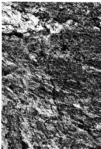
Photo. 6. Shale and the broken chert in the fracture zone at west side from the fault.
