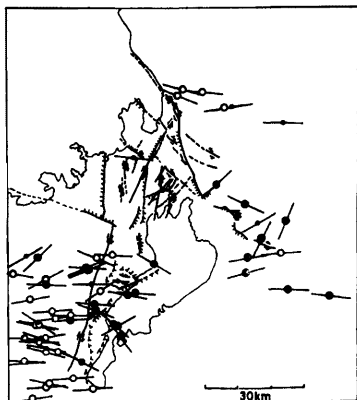
Fig. 8. Relation active faults distribution and earthquakes mechanism, open circle; quadrant type, solid circle; thrust type, solid line: direction of principal stress.
