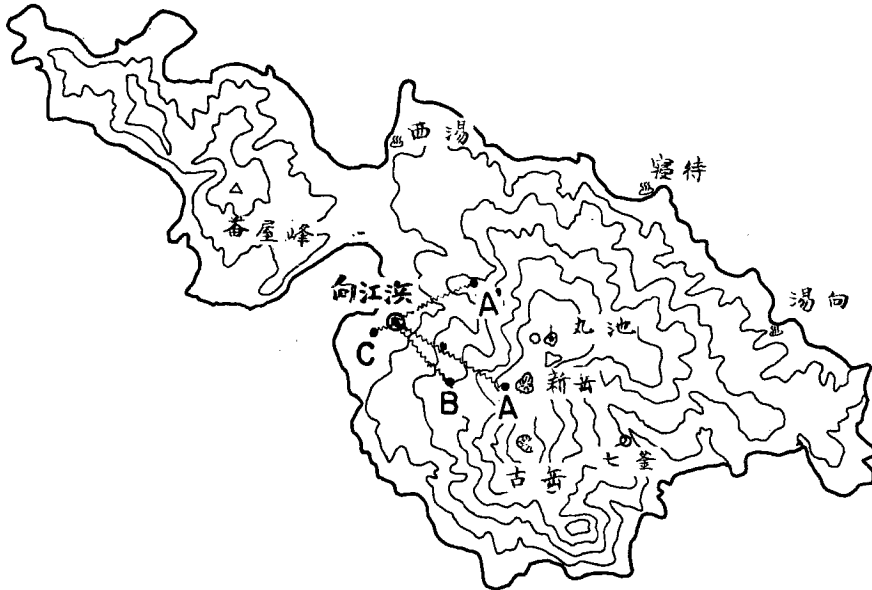
Fig. 4 A net of seismic observation. ● : Base station • : Positions of seismometers
