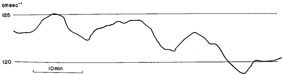
Fig. 3 Velocity variations in the river with the averaging period 5 min. B=100 m, H=2.1 m, \bar{u}=1.23 m/sec.
