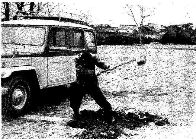
Photo 1 The method to generate SH-waves
