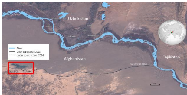
Fig. 2. Current stage of the canal construction. The spill seen in the middle marked by red square. Source: Landsat 8-9 (2024.01.20)
