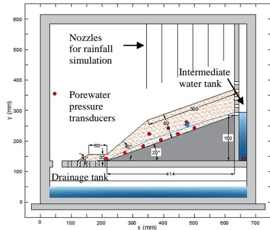
Fig. 1 Schematic diagram of the centrifuge container
