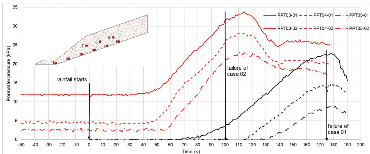
Fig. 2 Pore water pressure distribution of Case (i) and Case (ii)
