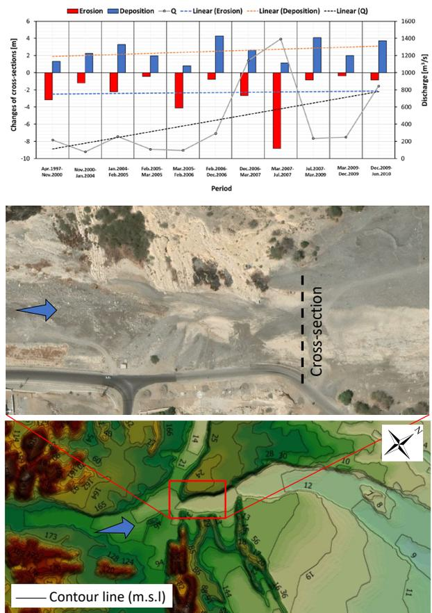
Figure 2. Dry channel bed level changes for multi cross-sections surveys from 1997 to 2010 catchments at the downstream of Wadi Samail
