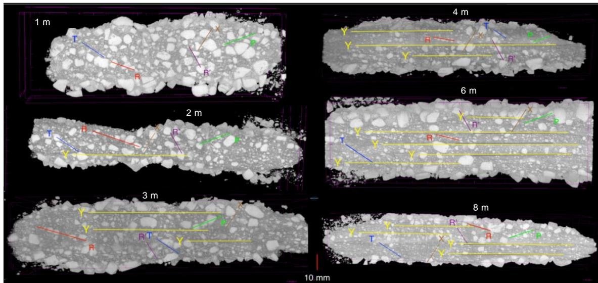
**Fig. 4.** Six types of Riedel shear structures can be recognized in terms of different shear displacements (1, 2, 3, 4, 6, 8 m) in this study. One interval in all the three-dimensional magenta boxes around the samples denotes 10 mm
