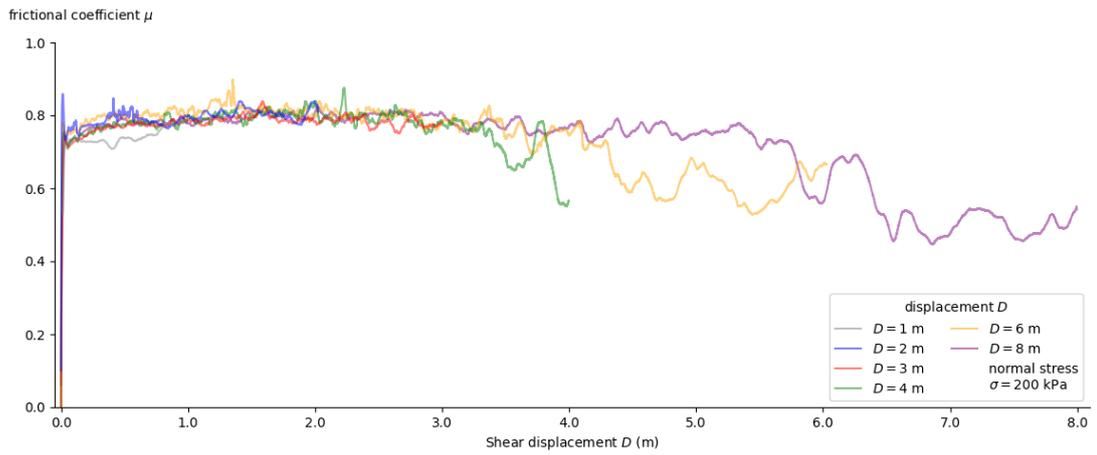
**Fig. 1.** The frictional coefficient in terms of shear displacement for different shear displacement tests.
