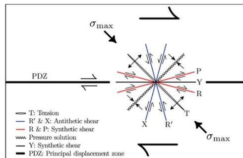
**Fig. 3.** An idealized Riedel shear system containing six types of shear structures (Xu and Ben-Zion, 2013).
