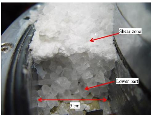
**Fig. 2.** View of shear zone formed in the test
