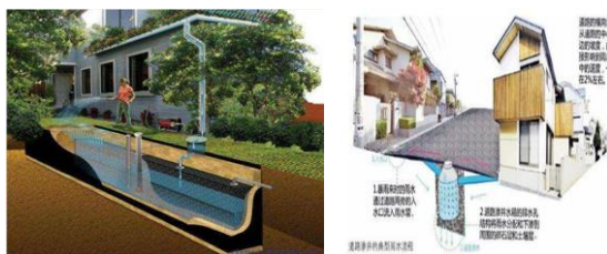
Figure 1 and Figure 2 on-site storage facility
